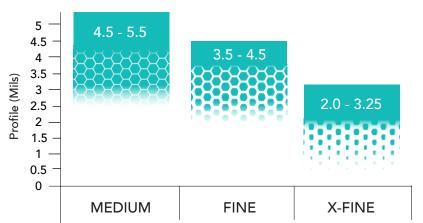
This guide shows the profile range of different grades of abrasives. The results were observed from a controlled environment using a standard blast cabinet system. The parameters of operation for the test were the following: 90-100 psi at the nozzle, nozzle to surface distance of 18", a 1/4" orifice venturi nozzle, on new 1/8" grade A36 steel, with a blast angle 75° to 105°. Results may vary depending on environmental conditions and equipment performance setup.
