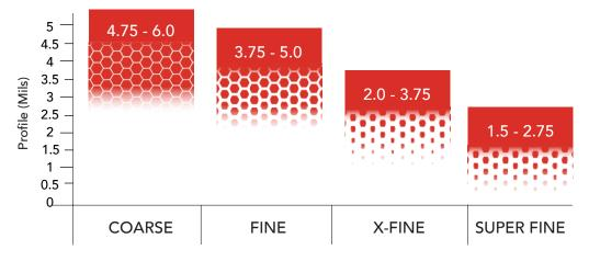
This guide shows the profile range of different grades of abrasives. The results were observed from a controlled environment using a standard blast cabinet system. The parameters of operation for the test were the following: 90-100 psi at the nozzle, nozzle to surface distance of 18", a 1/4" orifice venturi nozzle, on new 1/8" grade A36 steel, with a blast angle 75° to 105°. Results may vary depending on environmental conditions and equipment performance setup.
