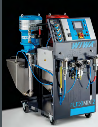
WIWA FLEXIMIX 2, electronic plural component spray equipment
